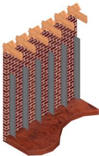
1. Attach metal studs to ceiling and floor in front of wall
